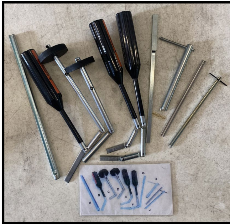
Figure 32. Elevator hoistway keys. These are left separated and stored within a small bag for use.
