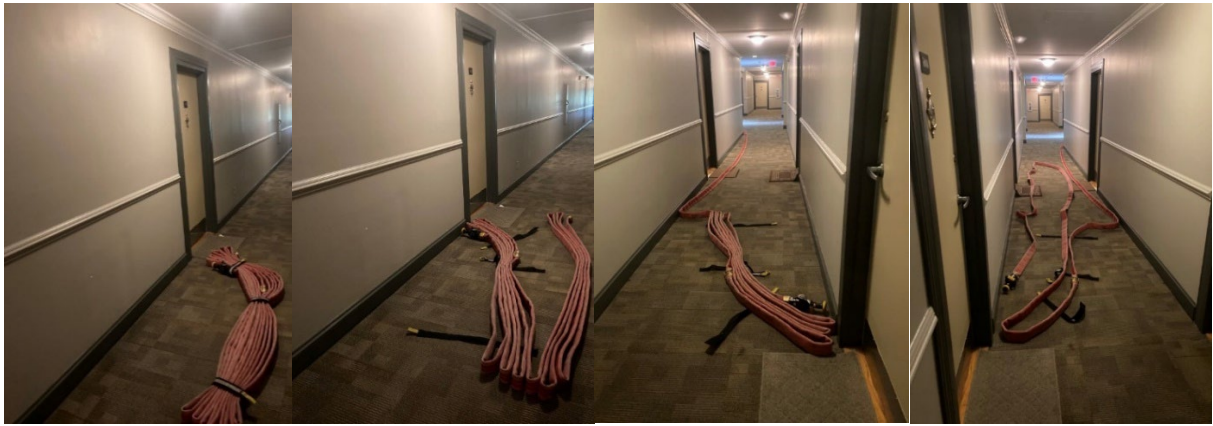
Figure 19. Reverse standpipe stretch in a clean hallway.
