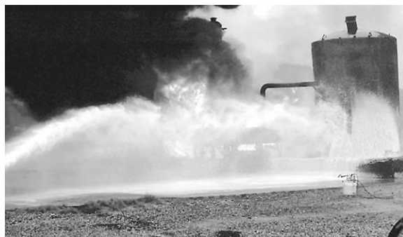
Figure 27: Rain-down method of foam application. 9
