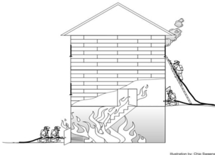
Figure 30. Hoseline positioning for a basement fire with an exterior entrance to the basement.
