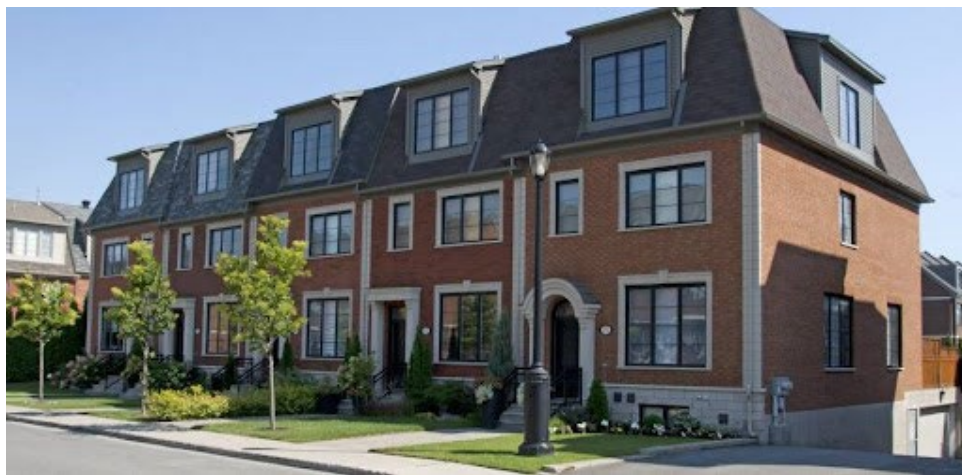
Figure 17. Example of a mansard roof.
