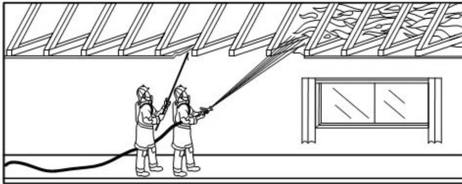
Figure 16. Projecting a hose stream into an attic.
