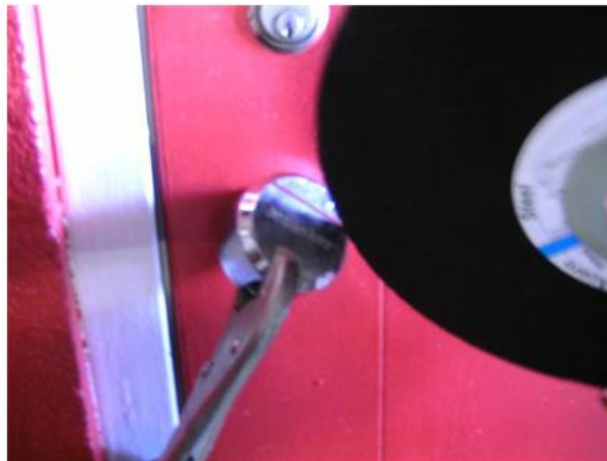
Figure 29: Cut hockey puck locks in the upper third portion.
