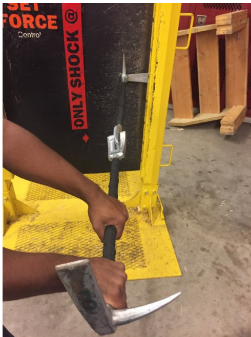
Figure 21: Pairing two Halligans together by the forks can provide additional leverage for forcible entry.
