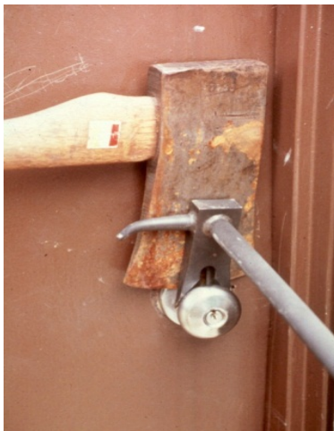
Figure 16: The use of a properly placed axe can provide leverage for prying.
