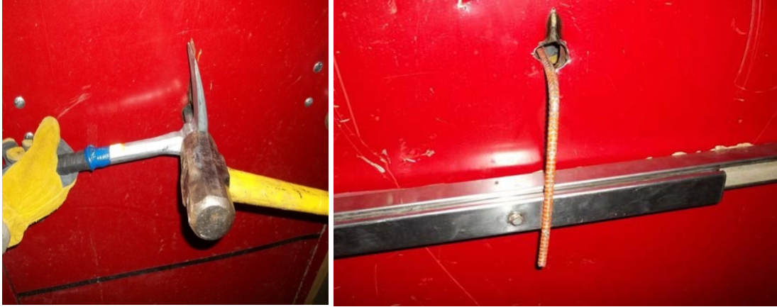
Figure 23: Creating hole in a door from the exterior close to the panic hardware is located (left) and placing the bent portion of rebar into the hole to pull on the panic hardware (right).
