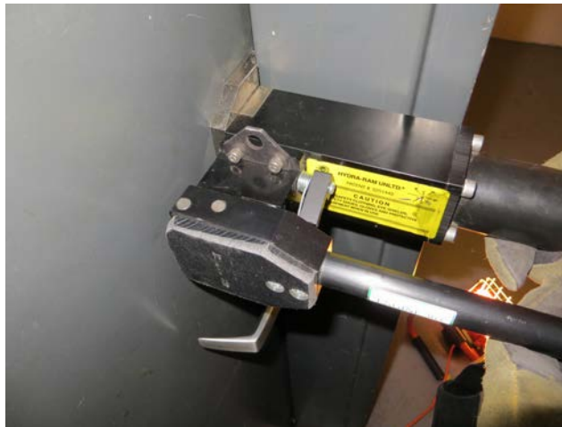
Figure 24: Using a hydraulic tool to force a door.
