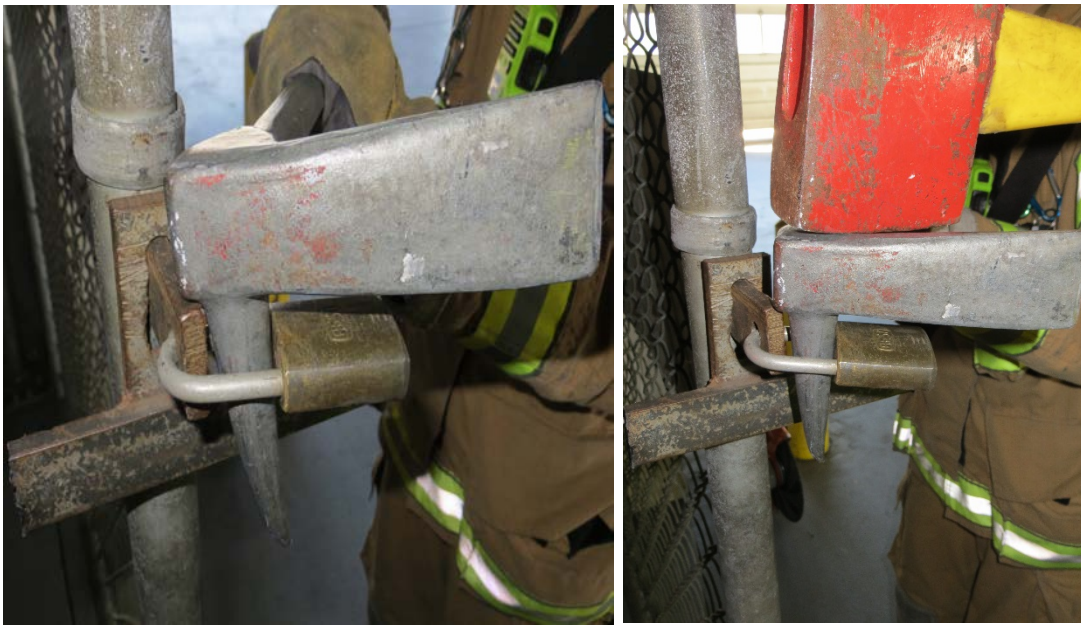
Figure 26: A Halligan bar and flat head axe are used together to force open a case hardened padlock.
