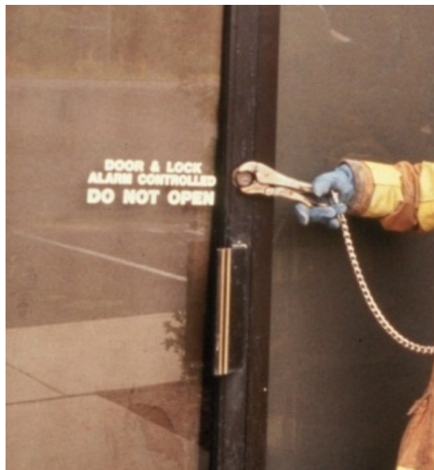
Figure 10: Unscrewing the lock cylinder with vise grips.
