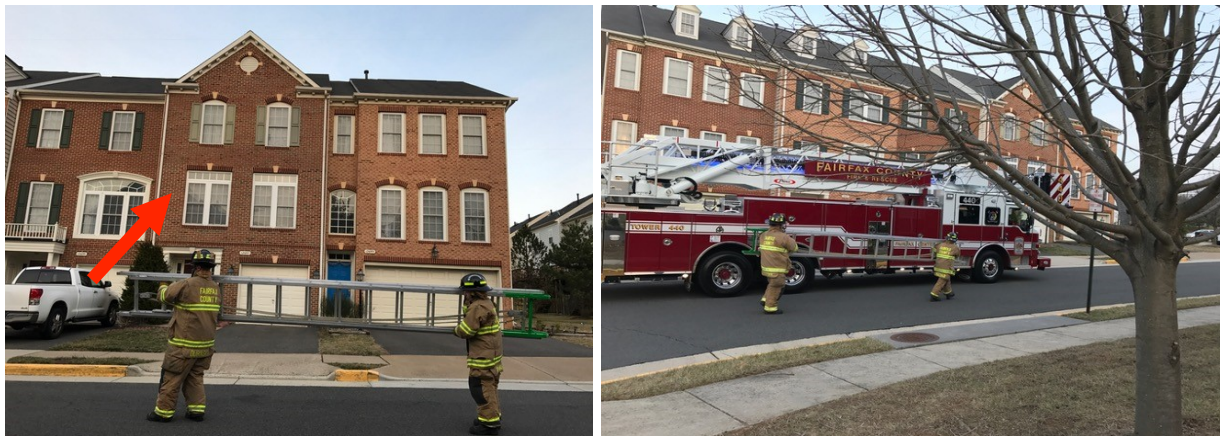
Figure 5: Heel-out storage means the ladder is directed toward the objective (left) and tip out storage allows deployment to an objective in front of the apparatus without turning the entire ladder (right).
