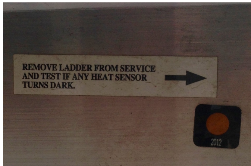
Figure 2: Personnel should inspect heat sensor stickers, if present, on their ladders for change of color and expiration during their inspection.
