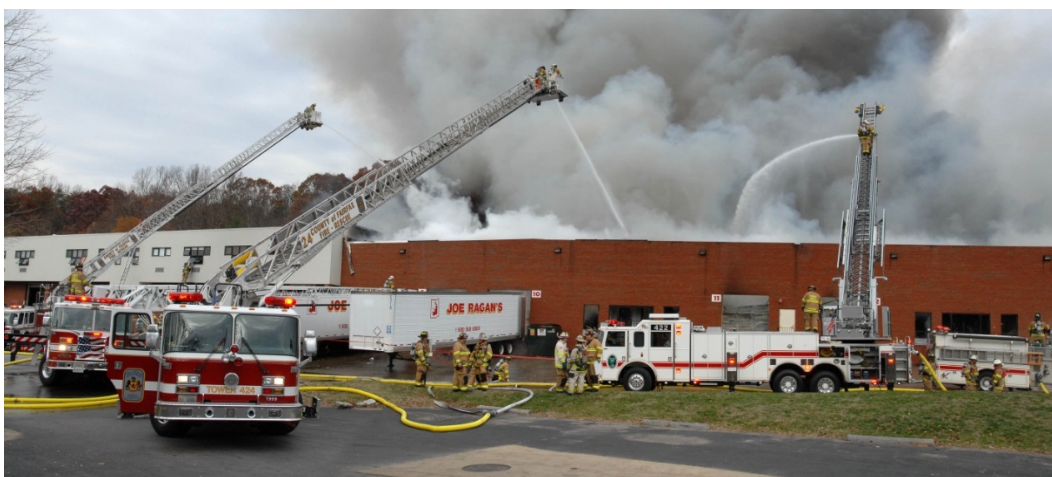
Figure 20: The use of elevated master streams can be very effective in large uncontrolled fires.
