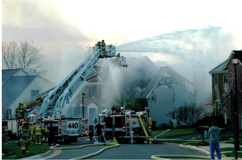
Figure 21: Elevated master streams on an aerial tower provides an effective tool in offensive exterior attack or for exposure protection.
