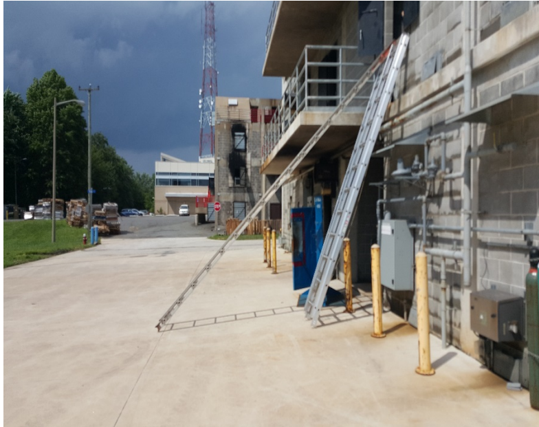
Figure 6: A 20-foot straight ladder versus a 24-foot extension ladder deployed to a second story window.
