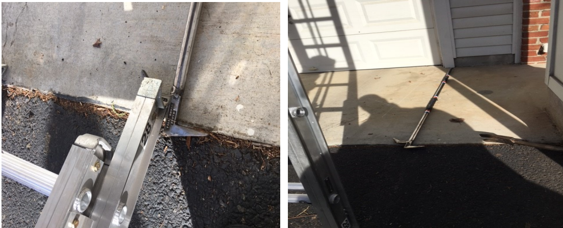
Figure 16: The use of a truck company hook to aid in heeling and placing it the correct distance from the building.
