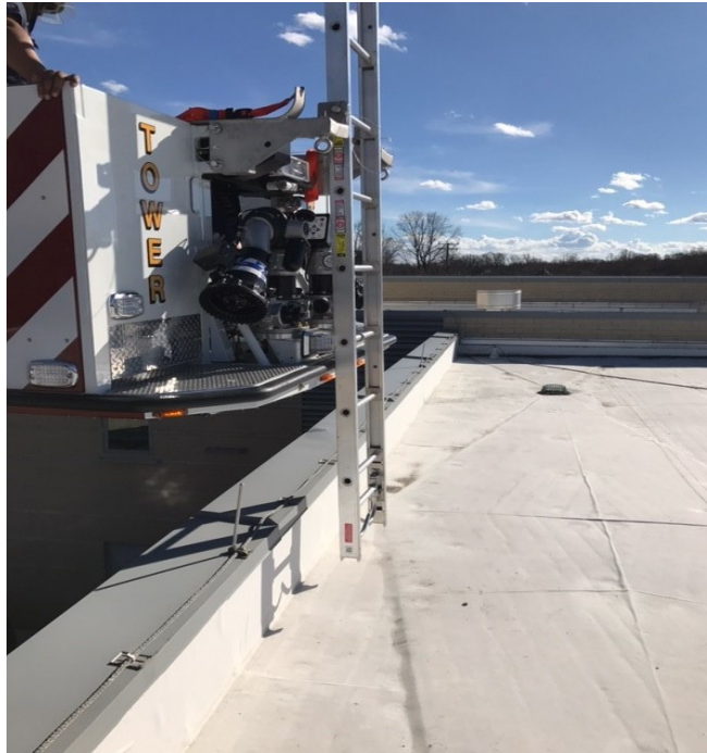
Figure 14: Ground ladder placement from aerial to access a roof with a high parapet wall. Some Tower Ladders have the factory installed option for this operation.
