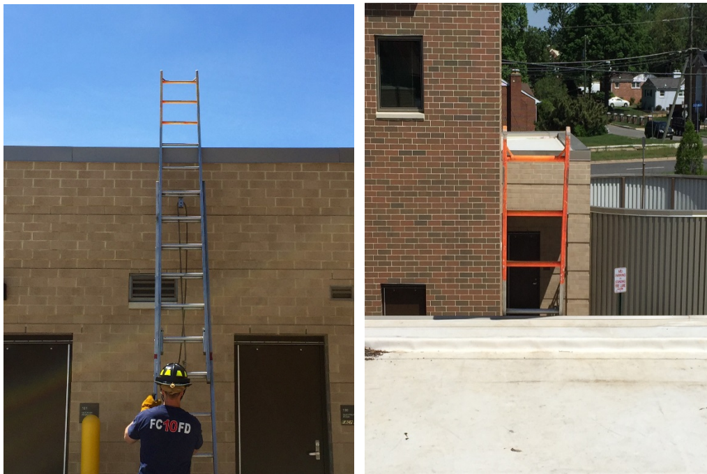
Figure 10: When laddering a roof, three to five rungs should be placed above the roofline.
