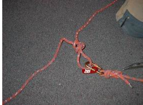
Figure 16: Additional search teams can deploy lines off a main line to increase the area covered by the search.
