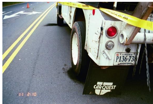
Figure 27: Vehicle that has come in contact with electric lines. Note the scorch marks below the tires.
