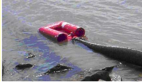
Figure 7: Floating dock strainer.
