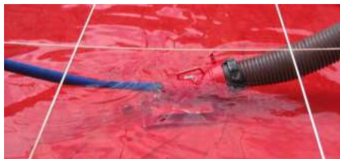
Figure 4: Low-profile jet siphon strainer.
